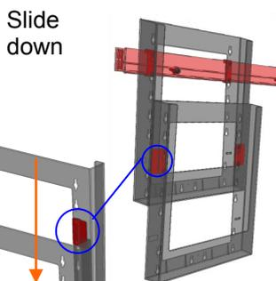
Down Joining Clips grip the face of the preceding pocket.
